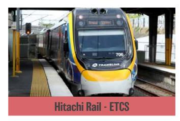
Cross River Rail is a new 10.2 km line that includes 5.9 km of tunnel under the Brisbane River and the CBD. SSL is supporting Hitachi Rail with the early works phase of CRR European Train Control Systems. ETCS L2 involves continuous supervision of train movement with continuous communication, which is provided by GSM-R, between the train and trackside.
